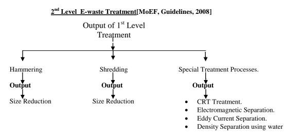
Fig: 10 Flow chart of 2<sup>nd</sup> level e-waste treatment.
