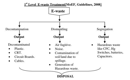
Fig. 9 Flow Chart 1<sup>st</sup> Level Treatment
