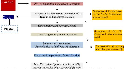
Fig: 11 Process Flow of type-CNT Dascu C-wastes Treatment [MoEF, Guidelines, 2008].
