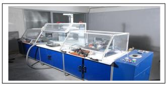
The internal phosphor coating from the inner side of panel glass is removed by using an abrasive wire brush and collected separately. The extracted air is cleaned through high efficiency bag-filter system to collect the phosphor dust. The phosphor dust so collected in the filter bags should be sent to TSDF.
