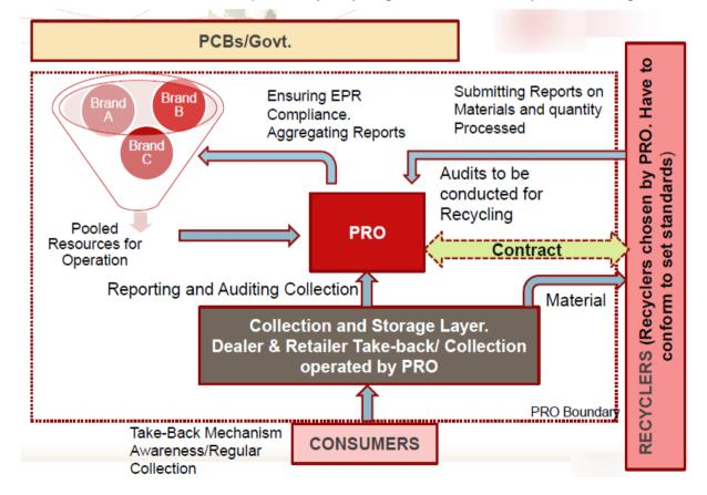
Figure 23: PRO functional diagram
