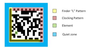
Figure 12: Anatomy of a Datamatrix Code
